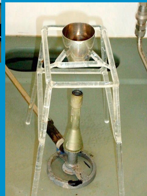
Calcination of 1-20 g on Bunsen in duplicate + crucible blanks
