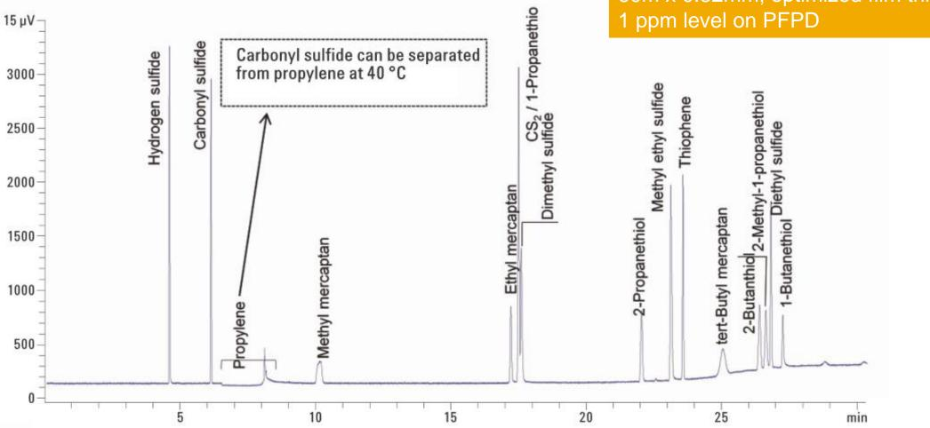
Select for Low Sulfur 60m x 0.32mm; optimized film thickness 1 ppm level on PFPD
