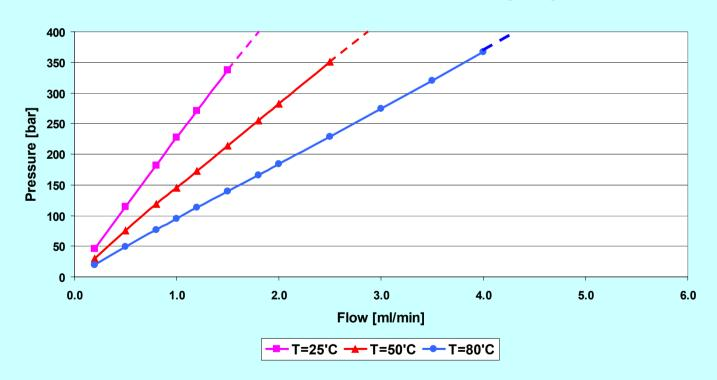
Column: SB-C18, 4.6 x 50 mm; 1.8 µm
