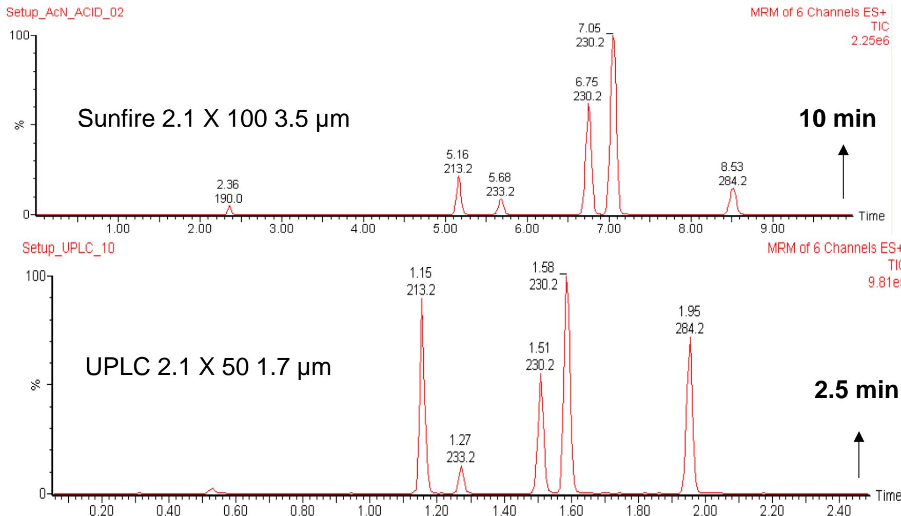
Sunfire 2.1 X 100 3.5um 10 ul injected partial loop VMW Pesticides Std 1 pg/ul
