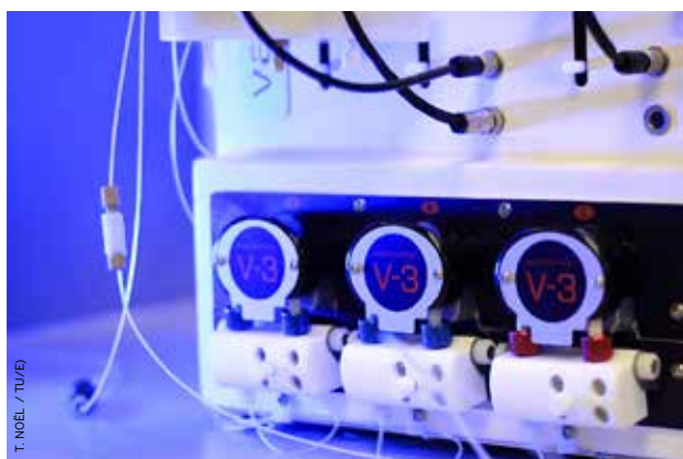
De flowreactor waarin wolfram CH-bindingen activeert.
